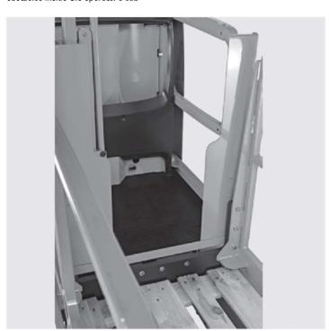
Simple and safe pallet entry with additional barriers in load direction
