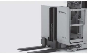
Optimal ergonomic order picking height at all times thanks to additional lift
