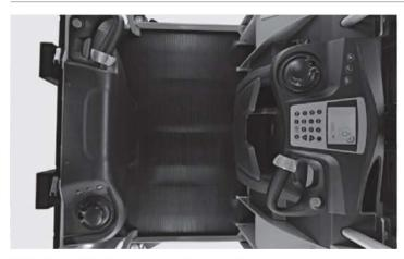
Efficient truck utilisation thanks to optional two-sided operation
