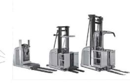
The king of order picking: the EK-X vertical order picker sets the benchmark in terms of performance, picking height, residual load capacity, functionality and ergonomics. The EK-X forges ahead into new dimensions of efficient goods handling with driving speeds of up to 13 km/h and lifting speeds of up to 0.4 m/s.
