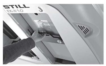
Simple lateral battery change optionally available, and electronic monitoring of battery locking for more operator safety
