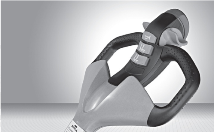
Tangibly better: control elements can be easily differentiated by their tactile characteristics
