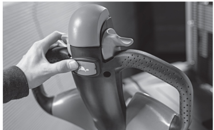
Precise in all situations: the optional creep speed switch enables manoeuvring in even the tightest spaces
