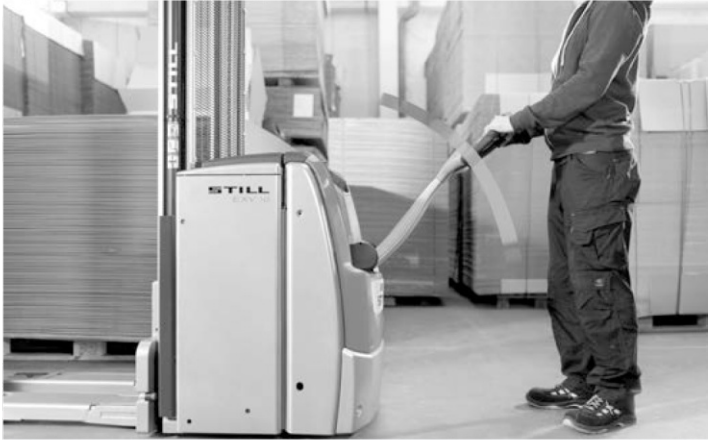
Safety in production: depending on tiller angle, speed is automatically adapted to the distance between the operator and the truck
