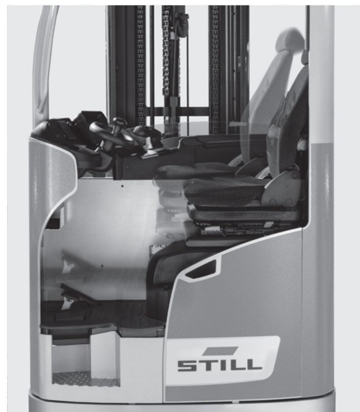
Ergonomically optimal position thanks to proportional adjustment of seat and footplate
