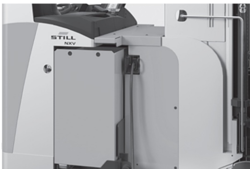
Optional opportunity charging access for lithium-ion batteries
