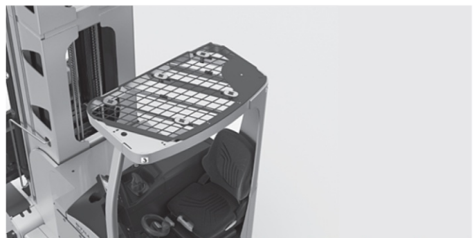
Whatever the application, we offer the right overhead guard, visibility-optimised, with or without metal or polycarbonate cover
