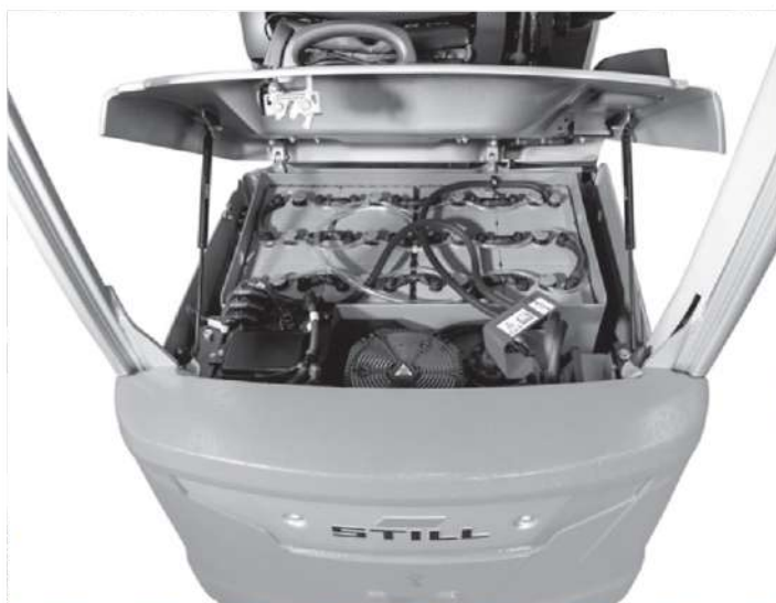
Both battery and drive are easily accessible - for maximum availability and convenient maintenance
