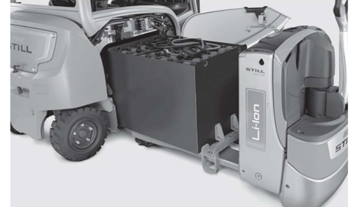
Battery change with electric pallet truck
