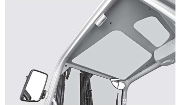
Enhanced visibility thanks to panoramic armoured glass pane
