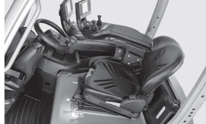
Swivel seat for comfortable reversing
