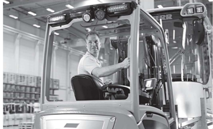
Swivel seat handle with optional horn operation for ergonomic reverse driving
