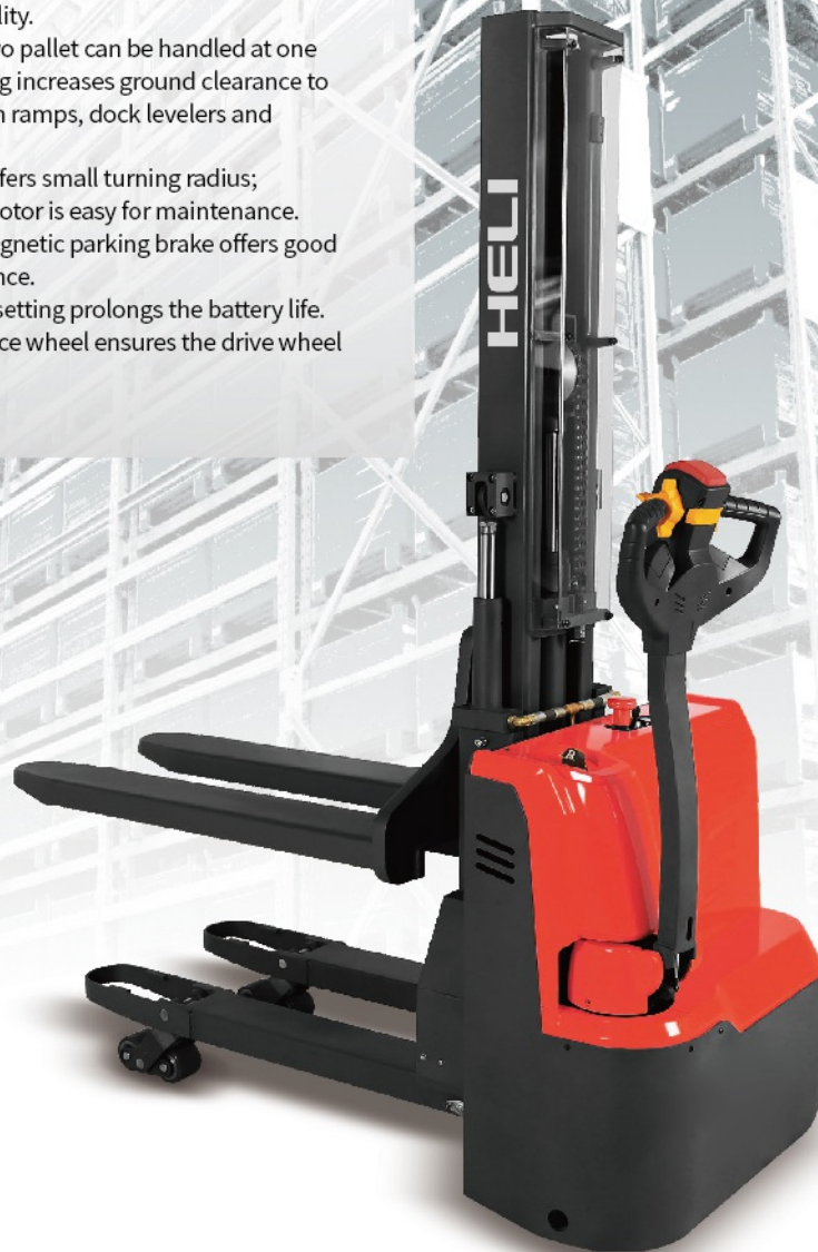
Compact design With very small turning radius, offer a range of application option in very confined space.
