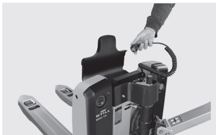
Always available: The integrated charger with Li-ion technology allows for convenient interim charging
