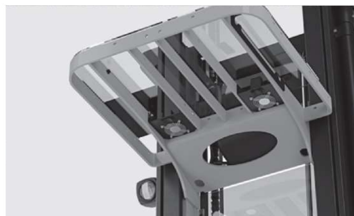
Optional fans on the overhead guard for a comfortable working temperature
