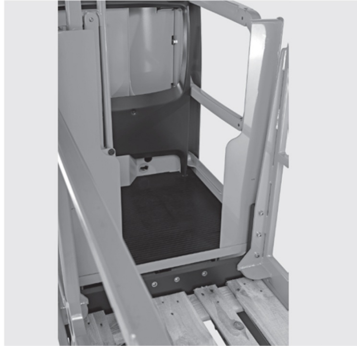
Simple and safe pallet entry with additional barriers in load direction
