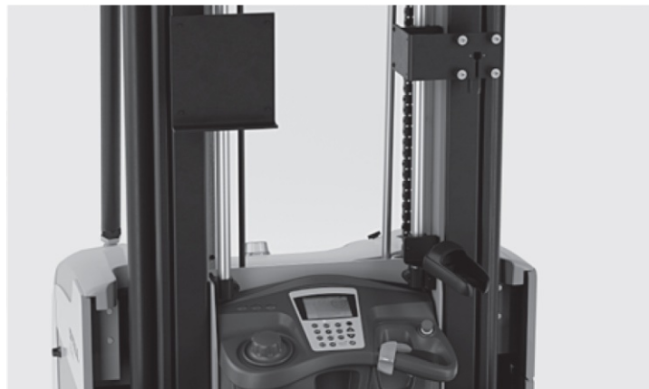
Optional operation with data terminal, printer and scanner
