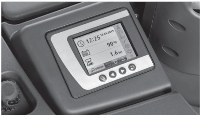
Everything in view: colour display with language-independent symbols shows all important functions
