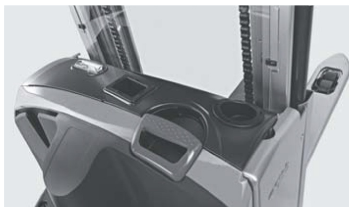
The steel battery cover is not only robust but also provides integrated storage options
