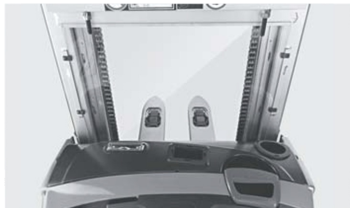
High handling capacity and best load visibility due to free view mast
