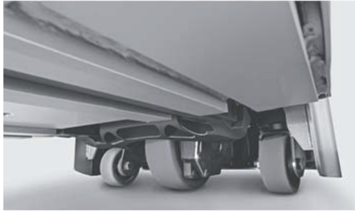
Up the ramp and down again: Traction in any situation due to the hydraulic support wheel suspension
