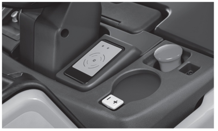
A variety of access options and a stand-on platform cushioning that can be adjusted by rocker switch (+/-)
