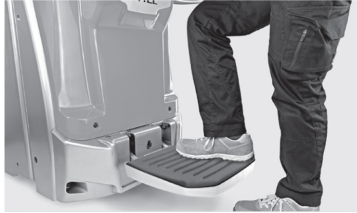
Adjustable side arms and air-sprung stand-on platform adjustable to individual driver weight
