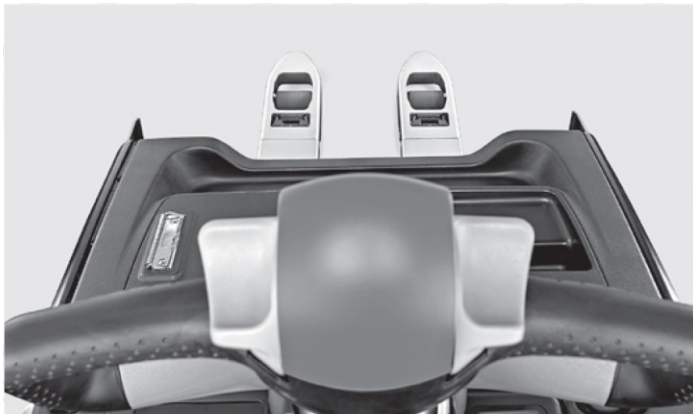
Optimum view of the fork tips allows a high and safe handling performance
