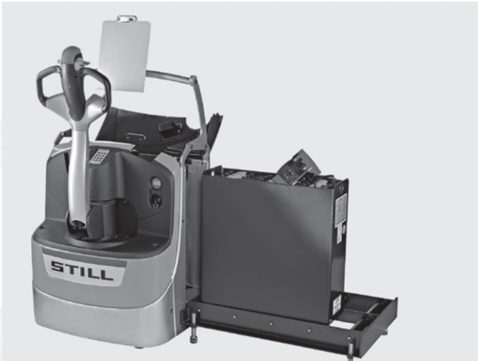
Maximum availability due to lateral battery change
