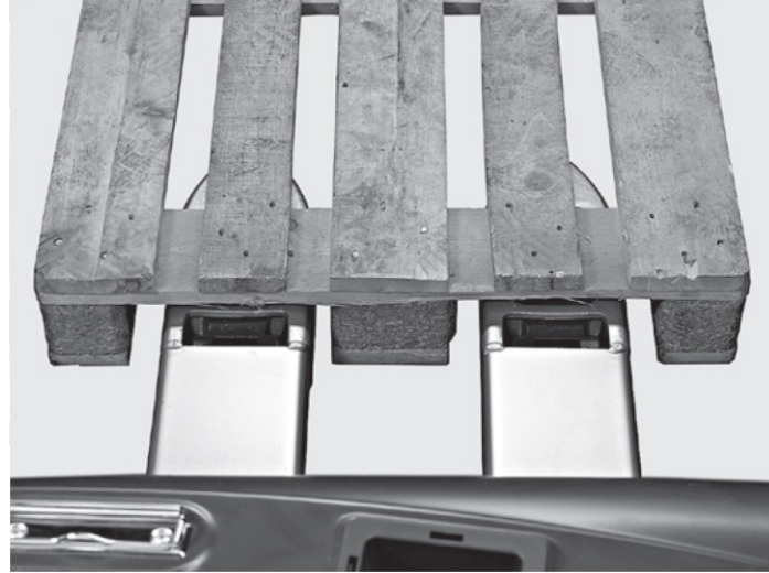
Optimum view of the fork tips for fast threading into the pallet
