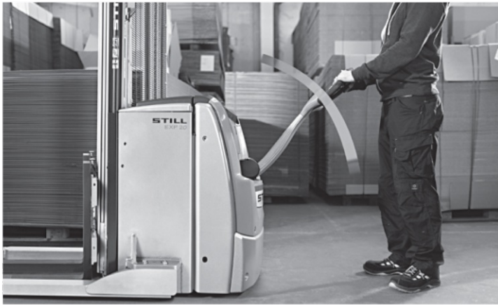
Safety as standard: depending on tiller angle, speed is automatically adapted to the distance between the operator and the truck (OptiSpeed) 1,2
