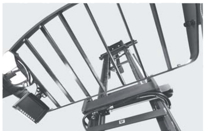
Optimised view through overhead guard
