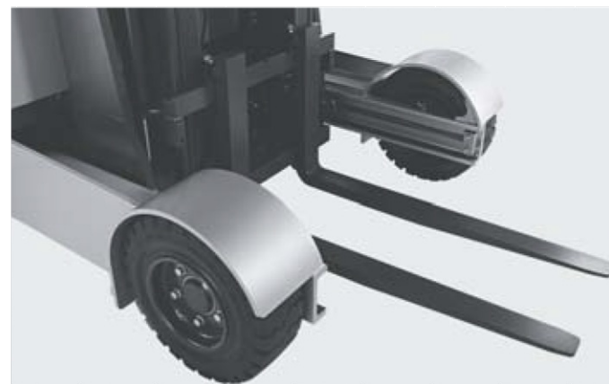
Super Elastic tyres with wheel protection for more security
