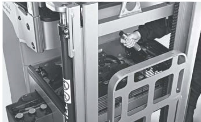
Standard lateral battery change for maximum availability and ergonomics
