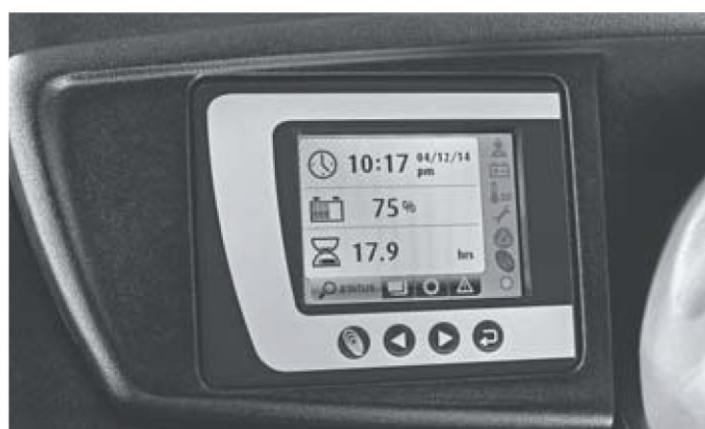
Colour display and control unit shows battery status, direction of travel and additional information
