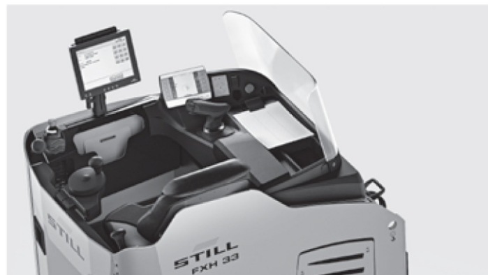
Easy positioning of optional data terminal and other accessories thanks to integrated accessory rails
