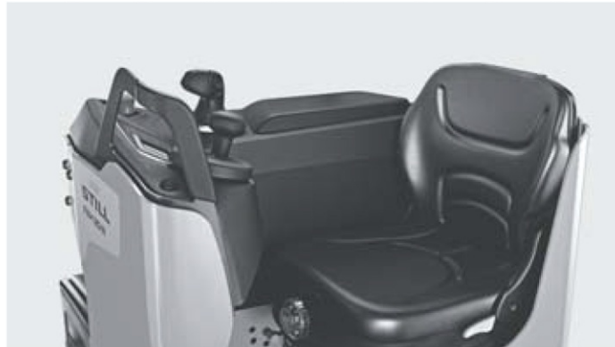
Cushioned driver's seat which can be adjusted to the driver's weight for maximum comfort
