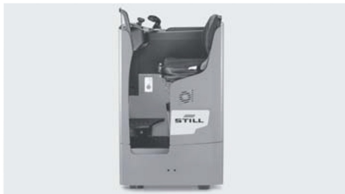
Height-adjustable foot plate for individual operator adjustments
