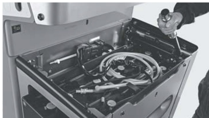
Standard lateral battery change for maximum availability and ergonomics
