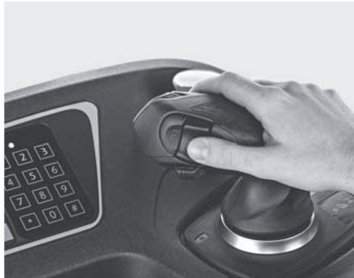
Individual operation thanks to optional Joystick 4Plus for lifting, lowering and transmission control without having to change hands
