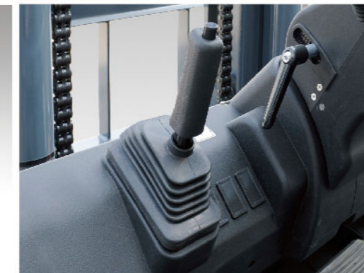
Ratchet type parking brake
