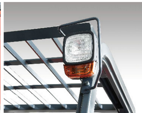
LED signal (standard configuration)
