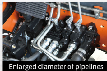
Enlarged diameter of pipelines
