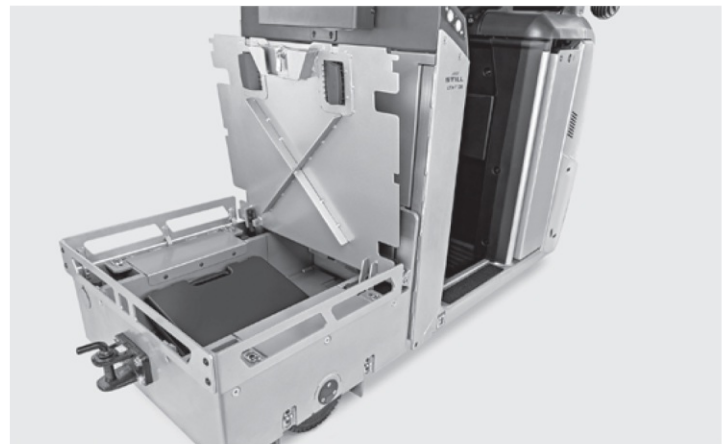
Storage compartment in the transport platform 3
