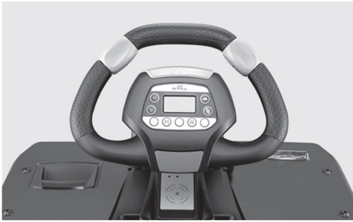
Unique STILL Easy Drive steering wheel for optimised driver control and operation of all functions without changing grip 2
