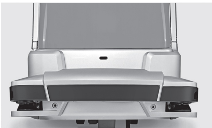
360° personal protection provided by integrated safety laser scanners in the LTX 50 iGo systems
