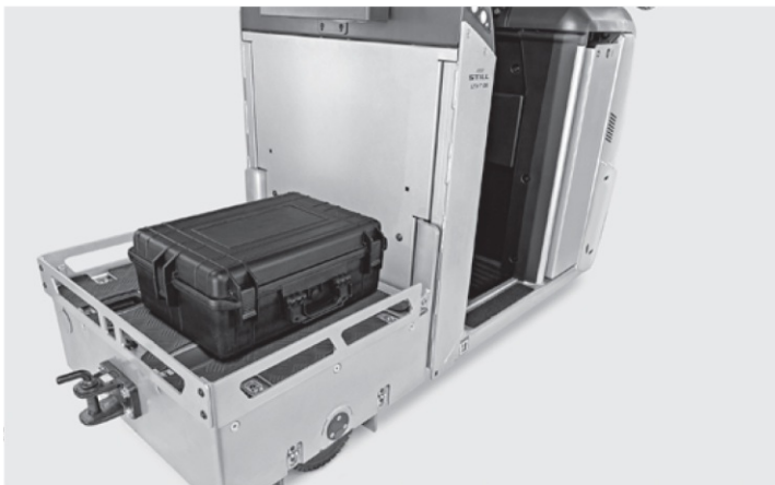
Storage surface with lashing eyelets for up to 600 kg 3
