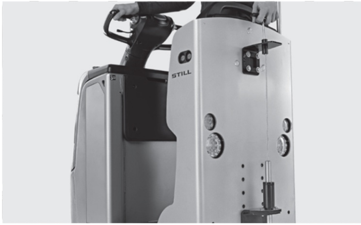
Fast release of coupling from driver's seat 1
