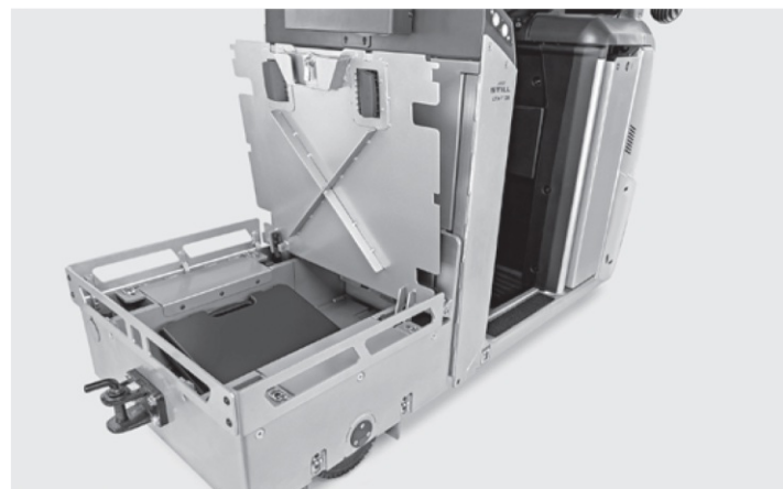
Storage compartment in the transport platform 3
