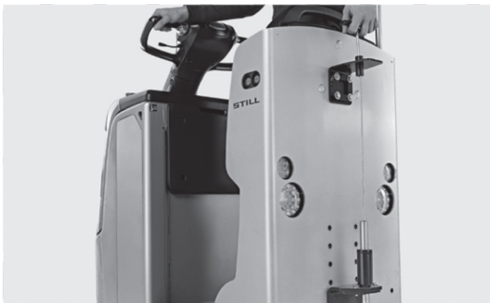
Fast release of coupling from driver's seat 1
