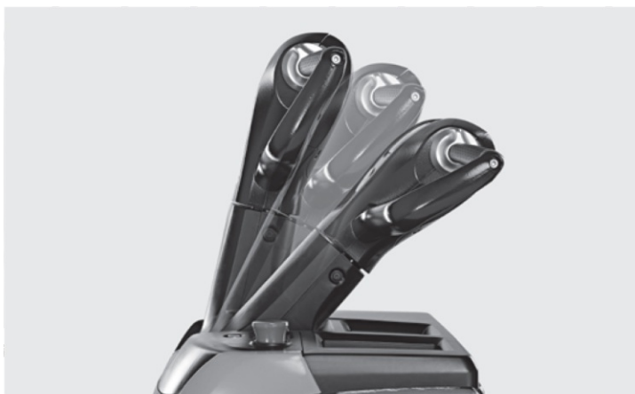
Height-adjustable steering for different drivers 1
