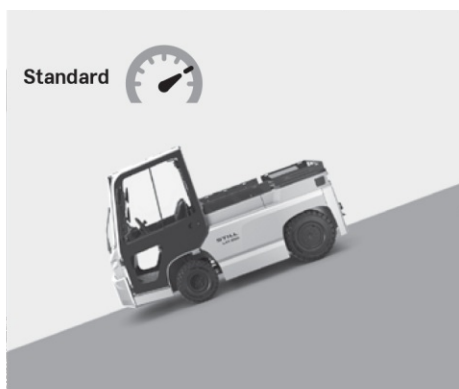
Basic: previously set speed on descent is manually limited via the switch.
