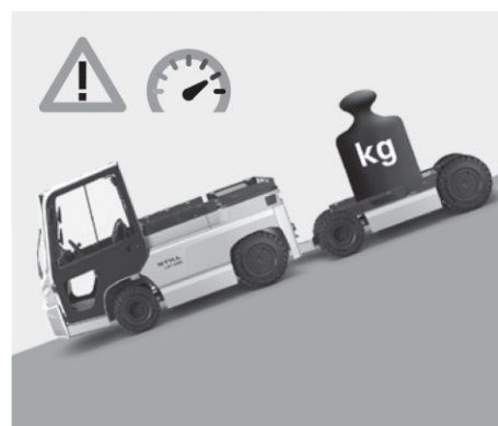
Premium: gradient shown on the display, speed reduction depending on load and gradient.
