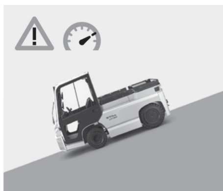
Eco: gradient shown on the display, previously set speed is limited to a predefined value when a gradient is detected.
