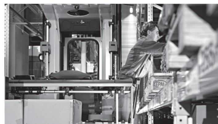
Tilting bar for ergonomic order picking to the last article on the pallet
