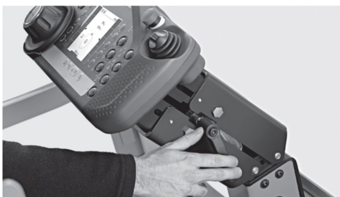
Three-dimensional positioning of the control panel
