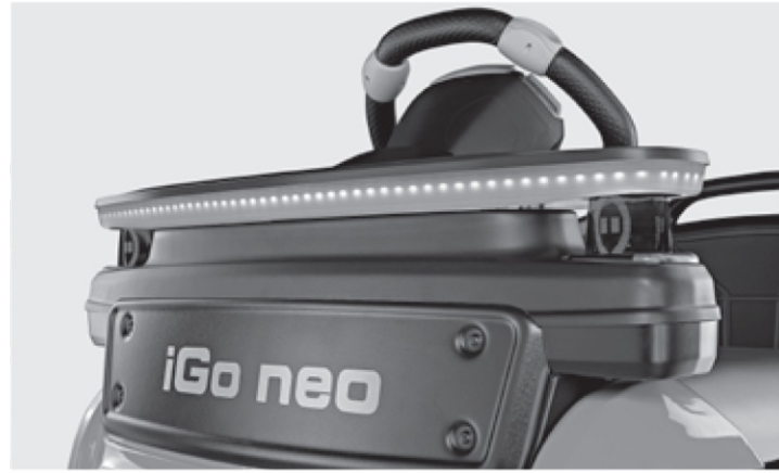
Always well informed: LED signal units indicate the current operating mode of the vehicle to the operator
