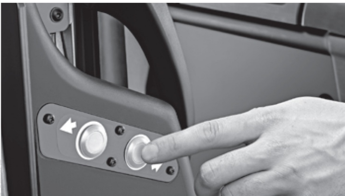
Double-sided pedestrian mode for improved handling even during high picking densities
