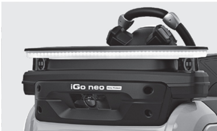
Safety in a new dimension: the optional 3D front camera of the OPX iGo neo detects obstacles over the entire vehicle height
