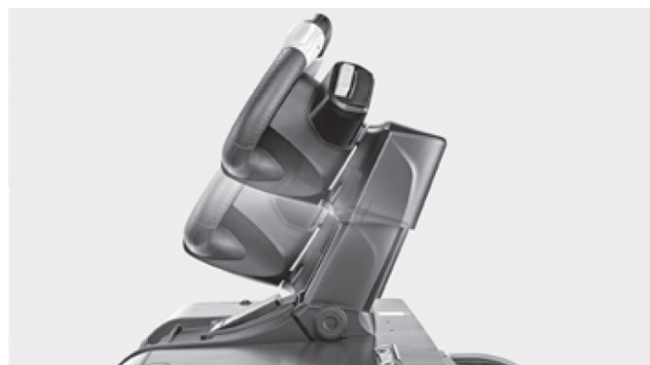
Maximum ergonomics due to the height-adjustable steering wheel and improved angle for individual driver preferences
