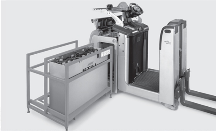
Always available thanks to lateral battery change
