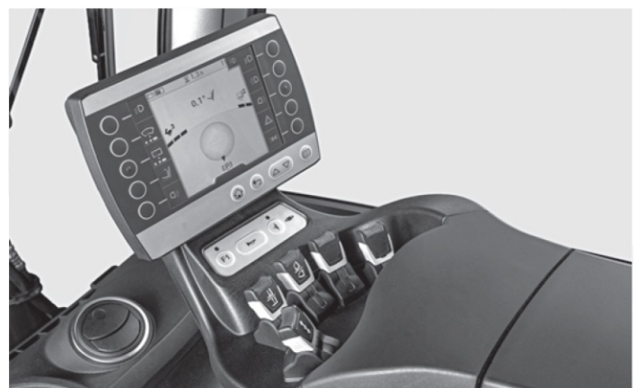
Safe, intuitive operation with the STILL Easy Control display and control module
