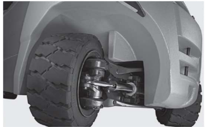
Manoeuvrable and stable high pendulum axle
