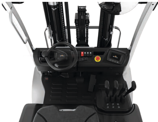
Flexible and comfortable: the operator's seat and steering column are infinitely adjustable, so that the cab can be quickly and easily adjusted for operators of different heights
