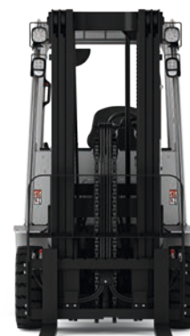
Keep everything safely in sight: the slim triplex mast allows for optimum visibility and lifts loads to heights of up to 6.55 metres
