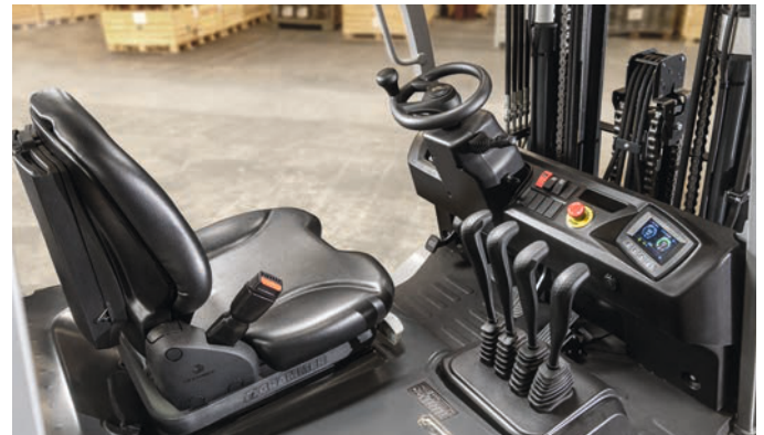
Good thinking: the elements of the STILL hydraulic operation are arranged so that they are convenient to use even when wearing work gloves
